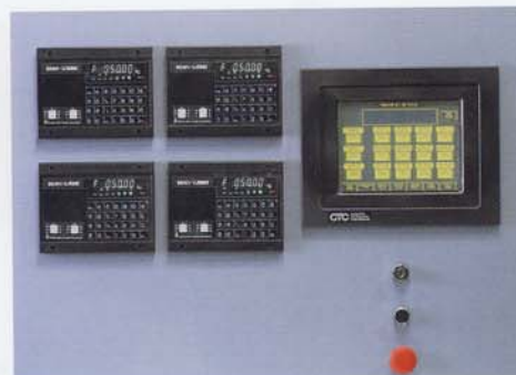
Four in-line packers are controlled from a central station.
