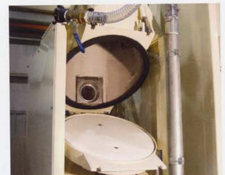
Stainless steel hopper has quick disconnect fittings and drop-down bottom for easy cleaning.
