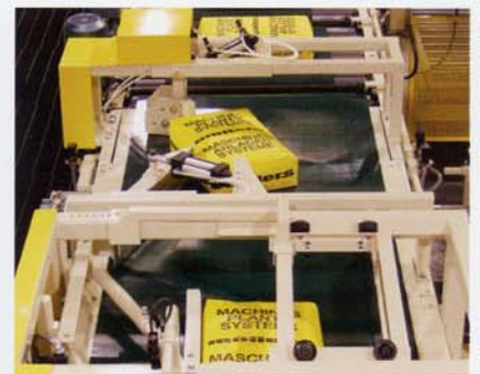
Bag turning post handles up to 50 bags per minute.
