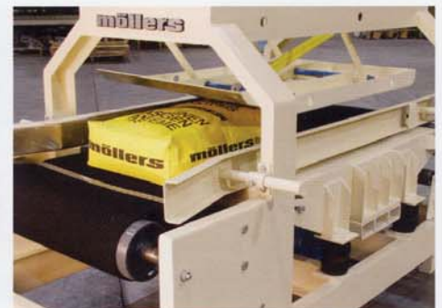
Bag equalizer flattens air-tight, sealed bags.
