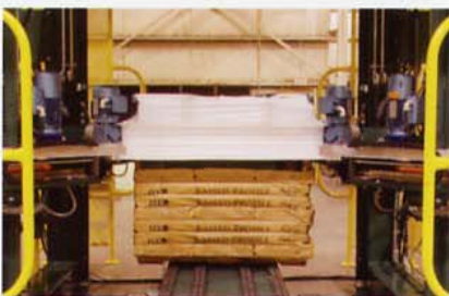
The hood is stretched over the load and secured to the pallet.
