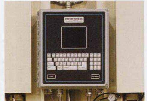
Packers can be quickly reprogrammed to handle multiple bag sizes and varying weights.
