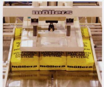
Layer squaring system and independent layer compressing plate square and flatten each tier.
