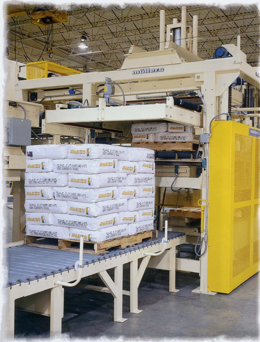
The standard empty pallet magazine holds 20 empty pallets.
