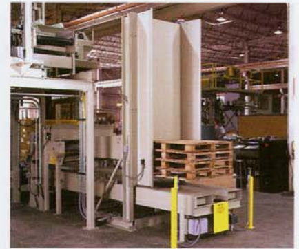
The standard empty pallet magazine holds 20 empty pallets.
