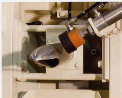
Nozzle with bag detection device.
