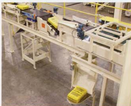
Automatic reject station kicks out under and overweight bags.
