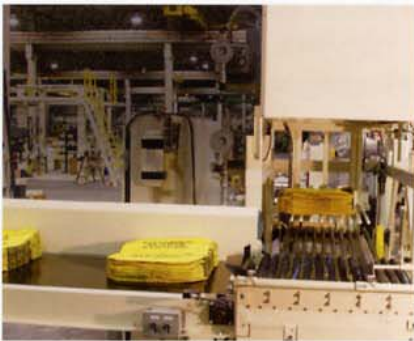
Conveyorized bag feeder provides a steady supply of bags to the packer.
