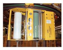
With it's rear opening film loading gate, the Octa-Thread film carriage allows for fast, easy and safe film threading.
