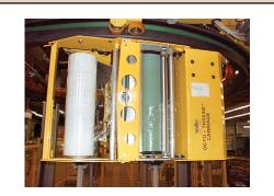
With it's rear opening film loading gate, the Octa-Thread film carriage allows for fast, easy and safe film threading.
