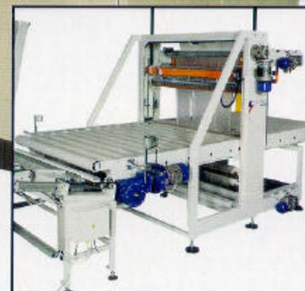
This device secures film to the load's upper and lower side before wrapping with stretch film. This kind of operation can be carried out using polyethylene film or air filled protective material.
